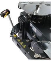
The new **Power Out** bead-breaking system allows you to comfortably manage each bead-breaking step via the ergonomic handle.
